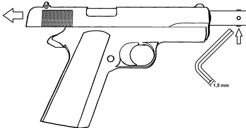
To adjust the laser a little to the left, for example, the right screw must first be unscrewed a little and then the left screw must be screwed in a little further. Make sure that neither of the two screws is screwed in or out completely. When adjusting in another direction, proceed in the same way.
